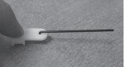
2) Rotate the wire so the Z bend wire is fully installed into steering link as shown.
